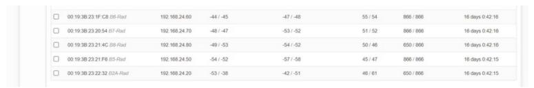
Signal levels range from -42dBm to -58dBm, averaging at -50dBm. The network manages to keep stable signal level for 16 days in a row.
