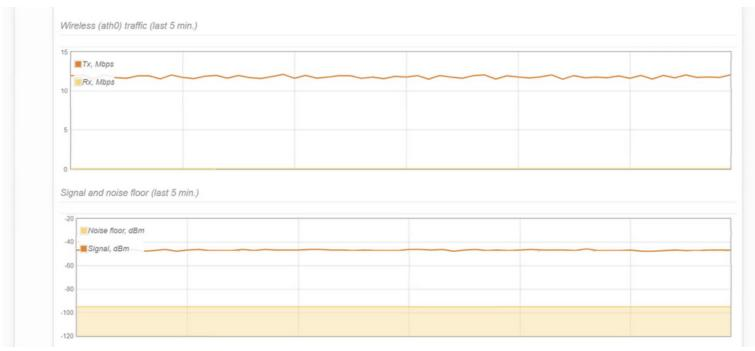
Real-time reports show that the internet connection is stable and without any drops averaging 13Mbps throughput, while the signal level stays stable at -50dBm.
